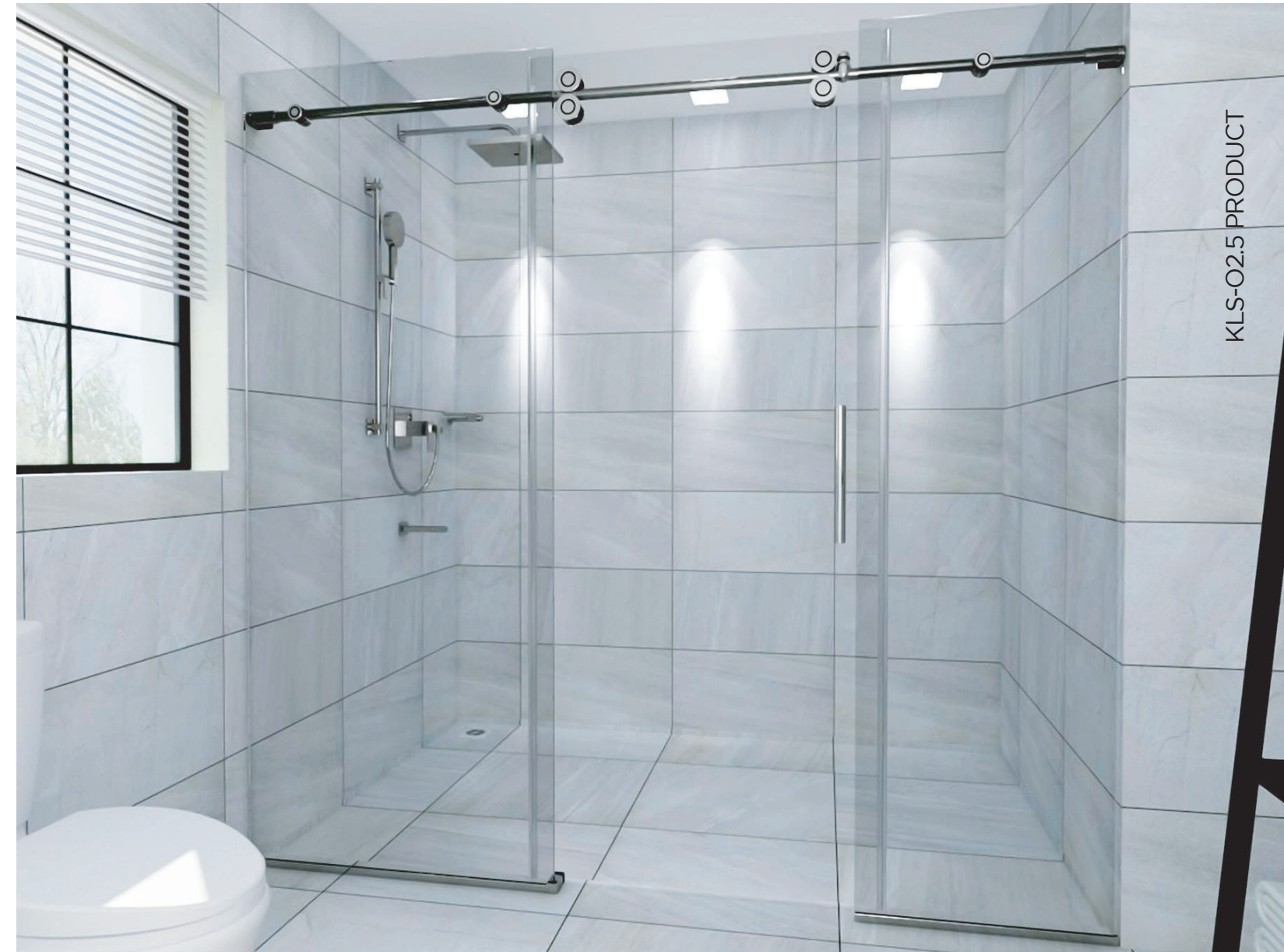
Layout 3 Sliding Door and two Fixed Panels to fit wide opening, 84" (2133.6mm) tall panels, for 3/8" and 1/2" (10mm and 12mm) tempered glass.
